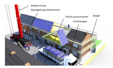
Figure 6:Fast retrofitting concept for roof of case 1.
